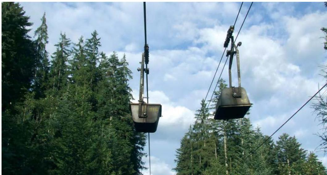
After sufficient deposits of gypsum were found in the mining area, it made sense to retrofit the freight ropeway for continued operations. The aim was to enable the ropeway to be operated for the next 30 to 40 years. The customer's goals were to reduce the number of people required to operate the system and to increase its efficiency. In addition, a new supply line from the Auermahd drive station was to be added.
